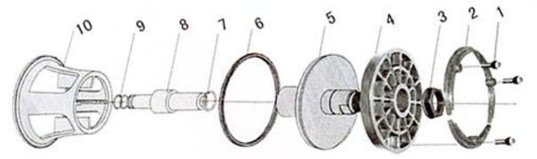
Retaining bolt 2. 3-piece retaining ring 3. Head nut 4.End cap 5.Supporting end cap plate
